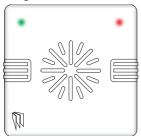
To set/unset the system using the external tag reader, present a pre-programmed tag to the centre of the device. The device will display the system status:
