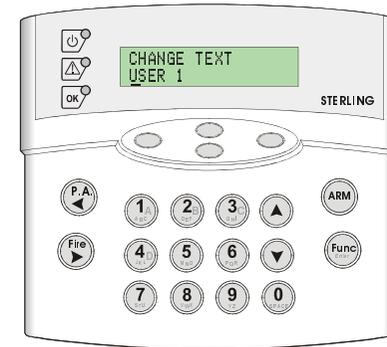
Use the scroll keys to display the change text options. You can change the following. When the required user is displayed the text can be changed by using the number keys 1 to 9:
