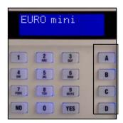
**NOTE**: For your security, the keypad becomes disabled for 90 seconds after 30 incorrect key-presses. It will subsequently be disabled again after 7 further incorrect key-presses. Once a correct code has been registered, the keypad is returned to normal operation.
