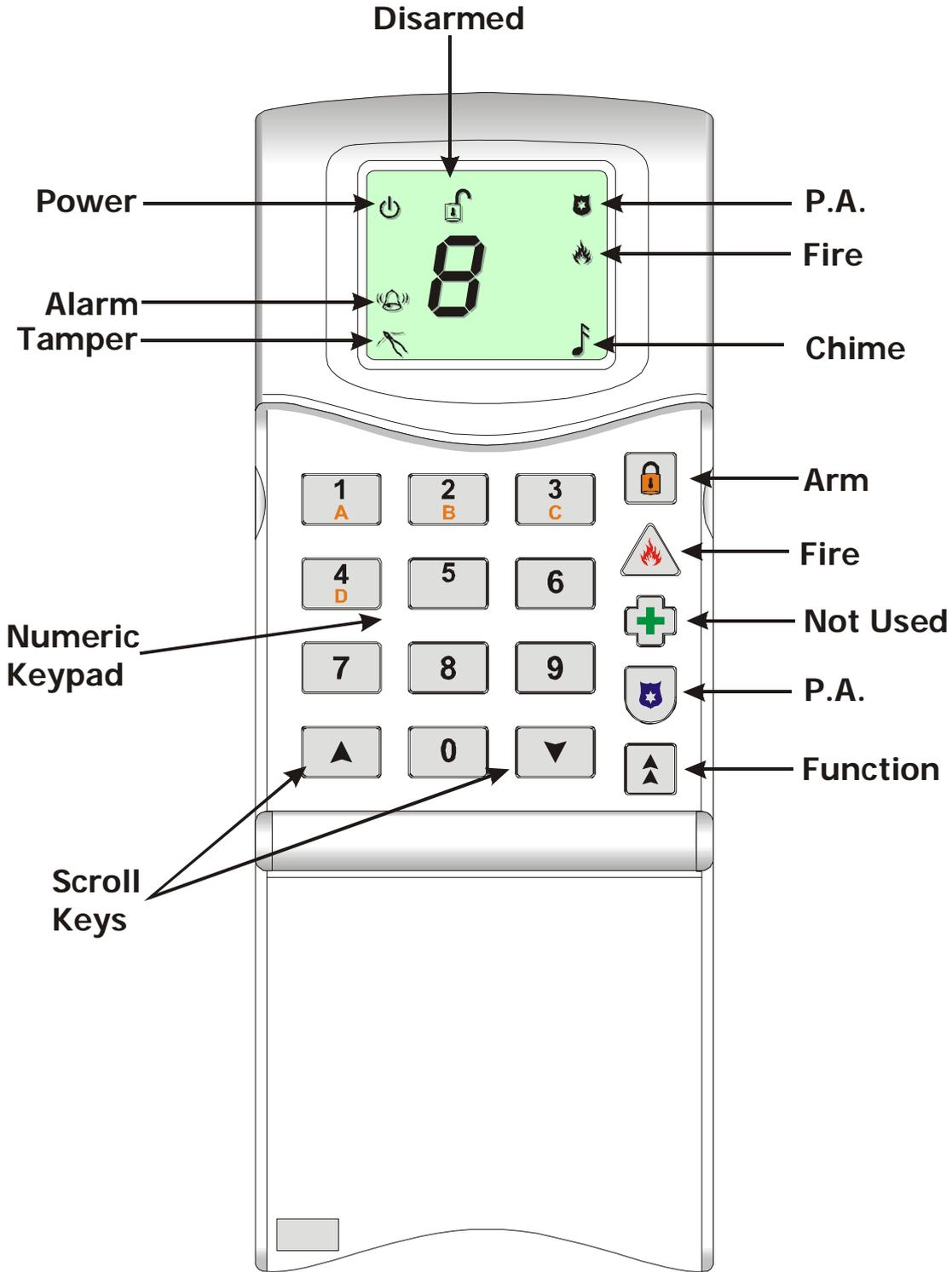
Whilst the keys and displays for both keypads differ, their functionality is very similar. Where functionality differs, methods for both keypads will be described. Where functionality for both keypads is the same, only one set of instructions for both are described.
